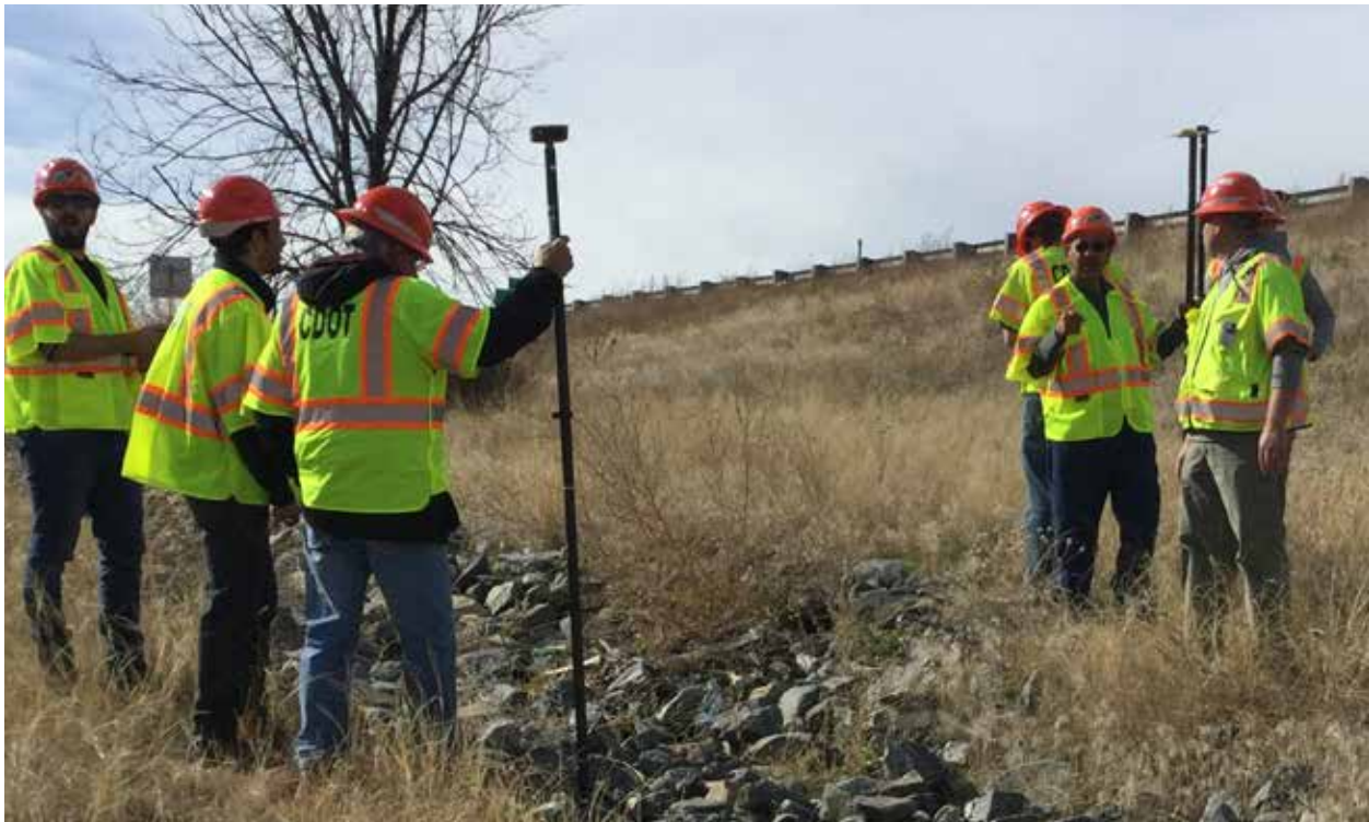
A field data collection training day for the CDOT Environmental Branch using ArcGIS Collector and the Geode sub-meter GPS receiver.
